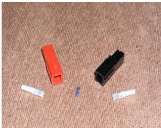
Components of a pair of Anderson Powerpole connectors: 2-silver-lined contacts, 1-red plastic housing, 1-black housing and 1-center pin.
