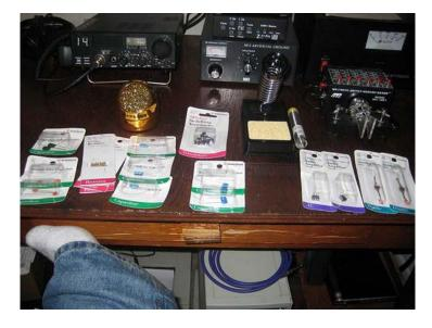
So far, I've laid out all the parts I'll need to build a Pixie II ORP transceiver for 40 meters. Right now I'm missing some inductors, the 40m crystal (sort of important) and some connectors. I'm going to pick those up at Trojan Electronics tomorrow -- where I probably should have gone in the first place instead of Radio Shack.
