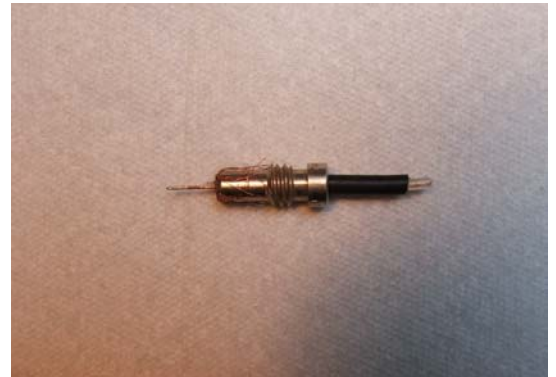
Photo 5- Shorted Center Conductor
