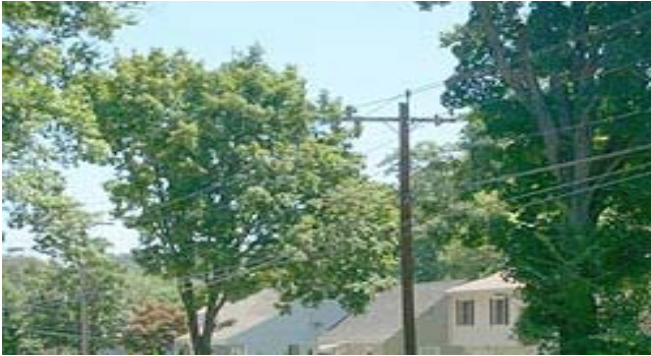
Broadband over Power Line (BPL) systems would use low and medium-voltage power lines like these to deliver broadband Internet service to homes and businesses.
