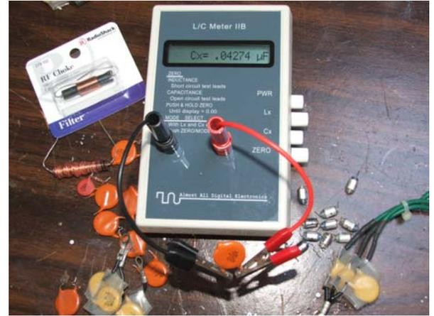
Here's the AADE LC Meter in action. The 0.05 uFd disc capacitor measures 0.04274 uFd
