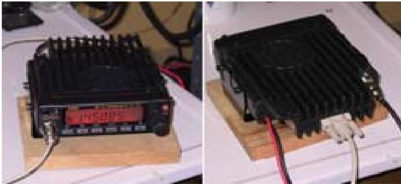
My Alinco DR-135TPMkIII wired for soundcard operations (left) and for packet radio operation (right).
