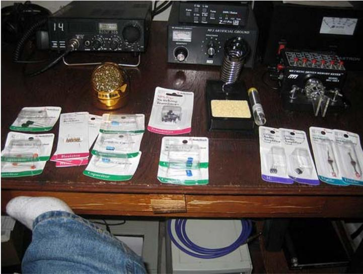
So far, I've laid out all the parts I'll need to build a Pixie II QRP transceiver for 40 meters. Right now I'm missing some inductors, the 40m crystal (sort of important) and some connectors. I'm going to pick those up at [Trojan Electronics](#) tomorrow -- where I probably should have gone in the first place instead of Radio Shack.
