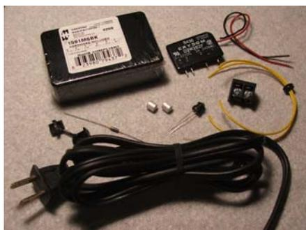
**Parts Used to Adapt relay**
